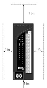
Make sure that there is a minimum of 2 inches clearance on the top, and 1 inch clearance on the bottom, each side, and in front of the *groov* RIO module, after it is mounted. Mount the module as shown in the diagram: with the Opto 22 logo at the top. Compliance with these guidelines helps ensure that the *groov* RIO module performs as described in the specifications.
