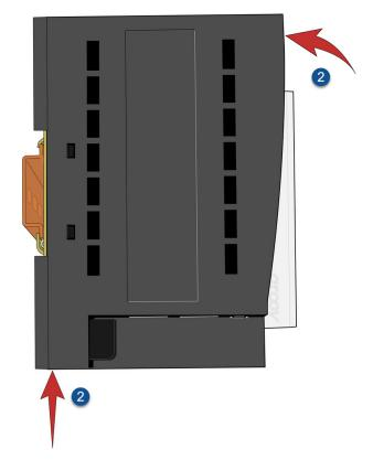
Before you release the module, verify that the top and bottom of the DIN rail adapters have engaged the DIN rail.
