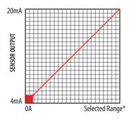
SENSED AMPS \*Factory calibrated ranges selected with the amperage range switch
