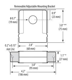
\* Terminal block may extend up to 1/8" over the height dimensions shown. \*\* Slide switch may extend up to 1/4" over the height dimensions shown.
