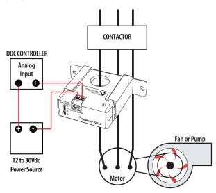
Note: This example diagram refers to the H721xC. Please see the H721xC and H921 installation guides for specific wiring information.
